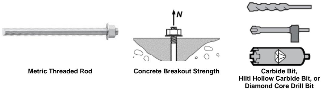
**TABLE 7—CONCRETE BREAKOUT DESIGN INFORMATION FOR FRACTIONAL THREADED ROD IN HOLES DRILLED WITH A HAMMER DRILL AND CARBIDE BIT (OR HILTI HOLLOW CARBIDE BIT), OR DIAMOND CORE DRILL BIT <sup>1</sup>**
